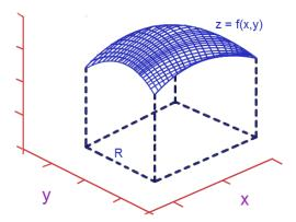
The figure above shows the graph of a function f(x, y) over its domain R where R can be any rectangular region  $R = [a, b] \times [c, d]$ . This notation means that the first variable, x, of the function takes values between a and b while the second variable, y, takes values between c and d. In this case the double integral can be denoted as
